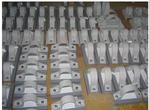
Fabricated pipe clamps for petro-chemical application.
